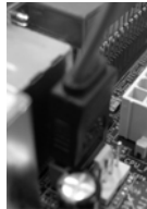
Connect the SATA data cable to the eSATAII connector (eSATAII_TOP)
