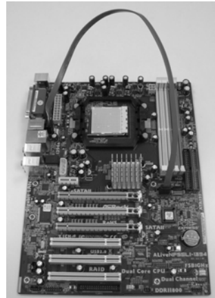
Connect the SATA data cable to the eSATAII connector (eSATAII_TOP)
