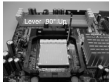
STEP 1: Lift Up The Socket Lever
