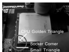
STEP 2 / STEP 3: Match The CPU Golden Triangle To The Socket Corner Small Triangle
