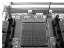
STEP 1: Lift Up The Socket Lever
