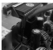
Connect the SATA data cable to the eSATAII connector (eSATAII)
