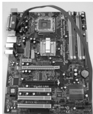
Connect the SATA data cable to the eSATAII connector (eSATAII)
