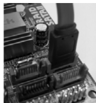
Connect the SATA data cable to the orange SATAII connector (SATAII_ORANGE (Port3))
