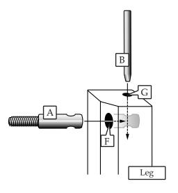
Place finger over **Hole G** (to keep **Pin B** from falling out) and turn leg upside down.
