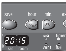
H: The TIMER indicator light indicates that the timer function has been switched on.
