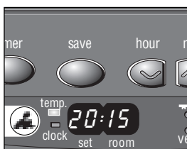
G: The required temperature on the left, the measured temperature on the right.
