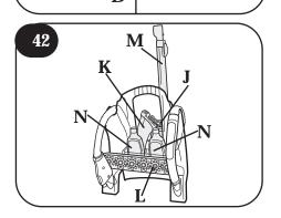
Place floor swivel tool (J), grout tool (K), brush assembly (L), telescoping wand (M) and detergent (N) into caddy as shown.
