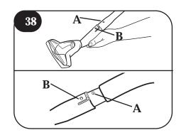
The handle must be in the upright position in order to get cleaning solution through the hose.
