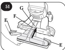
Return cleaner to upright position. Replace nozzle, making sure latches (E) are out.
