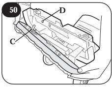
To replace brushes, align post (C) on brush block with hole (D) on bottom of cleaner. Turn brushes slightly until post fits easily into hole. Press brush assembly firmly to snap into place.
