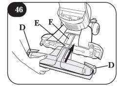
While holding nozzle in place, slide latches inward to lock in place.
