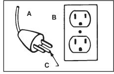
This appliance must be grounded. If it should malfunction or breakdown, grounding provides a path of least resistance for electrical current to reduce the risk of electric shock. This appliance is equipped with a cord having an equipment-grounding conductor (C) and grounding plug (A). The plug must be plugged into an appropriate outlet (B) that is properly installed and grounded in accordance with all local codes and ordinances.
