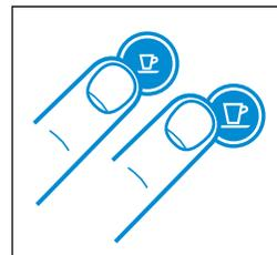
To turn the machine off before automatic Power Off mode, press both the Espresso and Lungo button simultaneously.
