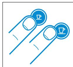
5. To enter the descaling mode, while the machine is turned on, press both the Espresso and Lungo button for 3 seconds.
