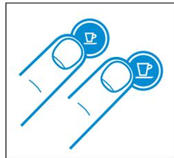
1. To enter the emptying mode, press both the Espresso and Lungo button to turn the machine off.
