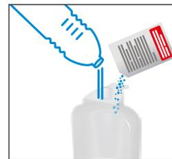
3. Fill the water tank with 0.5 L of potable water and add 1 Nespresso descaling liquid.
