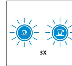
2. LEDs will blink fast 3 times to confirm machine has been reset to factory settings.
