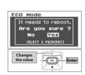
After it has restarted, the R-09HR will switch to ECO mode. While the R-09HR is in ECO mode, the indication " ECO " will be shown in the lower portion of the <Main Screen>.
