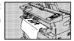
Set the original guide to match the original width and direction.
