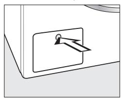
Press the drain pump access panel.
