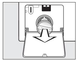
Remove the drain filter completely.
