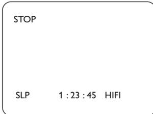
**3** While the counter is on the screen, press **CLEAR/RESET** to reset the counter to zero.
