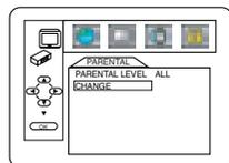
**6 Press the Number buttons to enter a four-digit password.** The password numbers will appear on the screen. Write down the password so you will not forget it. **Press OK.** The previous menu will reappear.
