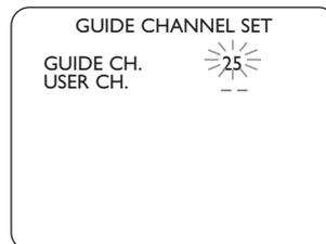
**6** Press the **Number** buttons, **▲**, or **▼** until the **User** channel number you want appears. If you have an antenna, choose channels 2-69. If you have Cable TV, choose channels 1-125. To select LI (line input), press 0,0 on the remote control.
