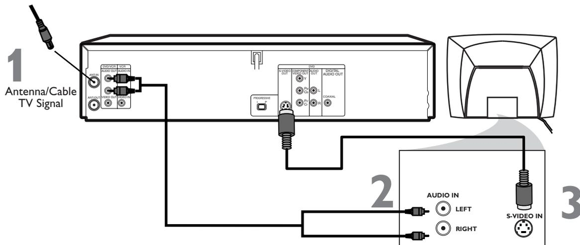
**1** Connect the antenna or Cable TV signal to the **ANT-IN (Antenna In)** jack of your DVD/VCR.
