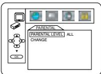
**7** Press **▲** or **▼** to select a level, then press **OK**. The rating levels continue on two menu screens. Press **▲** or **▼** repeatedly to move to the next or previous screen to find the rating level you want.
