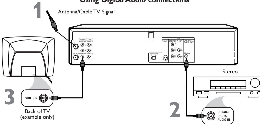
**1** Connect the antenna or Cable TV signal to the **ANT-IN (Antenna In)** jack of your DVD/VCR.
