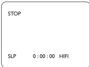
**4** When you later want to return to this point on the tape, press **DISPLAY** so you can see the counter (while tape play is stopped). Press ◀◀ or ▶▶. As the tape rewinds or forwards, watch the counter. When it reaches zero, press **PLAY** ▶ to play the tape.
