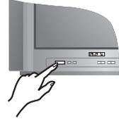
To switch on the set, press the on/off key. If the television remains in standby mode, press **P**
