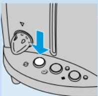
**1** When the toasting cycle has been completed, the bread carriage will be raised. If you wish to interrupt the toasting process, simply press the Cancel button.
