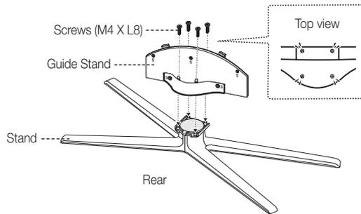
1. Connect the Guide Stand to the Stand using four screws (M4 X L8) as shown.
