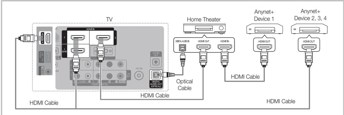
1. Connect the **HDMI IN (1 (DVI), 2, 3 or 4)** jack on the TV and the **HDMI OUT** jack of the corresponding Anynet+ device using an HDMI cable.
