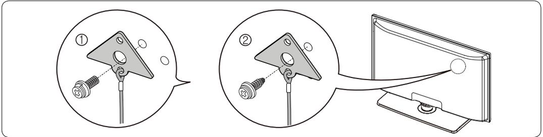
2. Firmly fasten the screw you provided (size M4xL20 or similar) to the wall or cabinet where the TV is to be installed.
