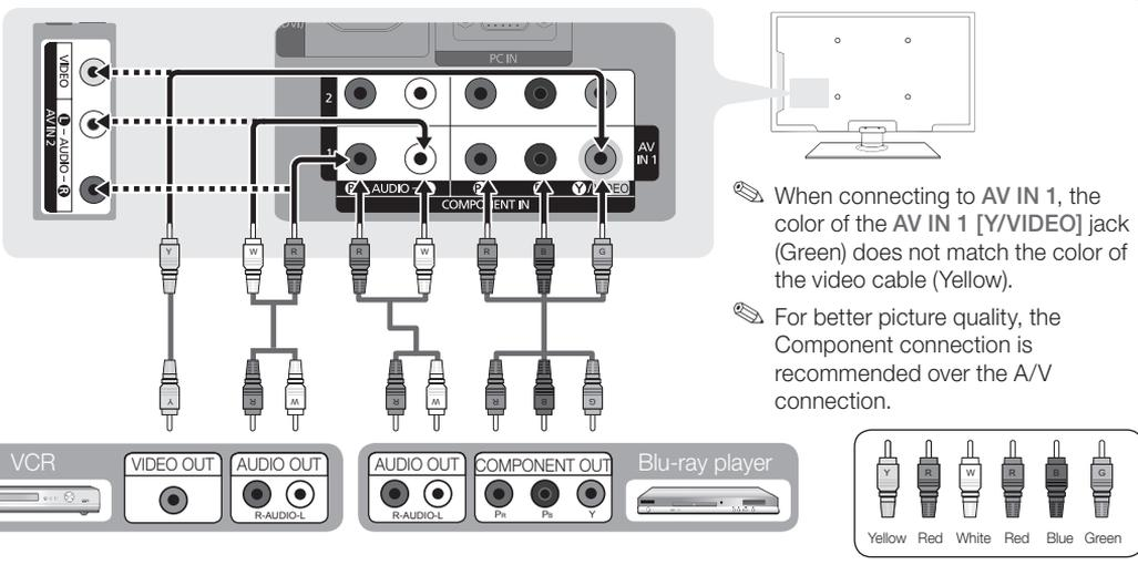
When connecting to **AV IN 1**, the color of the **AV IN 1 [Y/VIDEO]** jack (Green) does not match the color of the video cable (Yellow).
