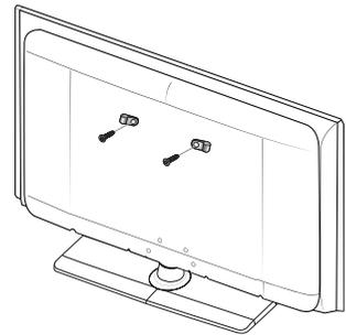
3. Connect the clamps fixed onto the TV and the clamps fixed onto the wall with a strong string and then tie the string tightly.
