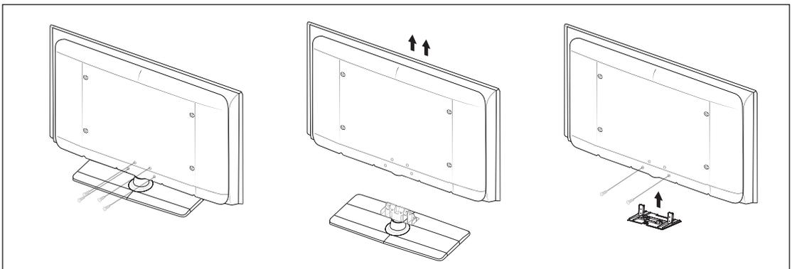
1. Remove four screws from the back of the TV.
