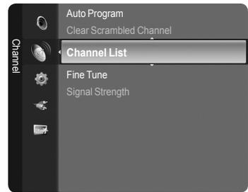
2. Press the **▲** or **▼** button to select the channel to be assigned a new name, then press the **TOOLS** button.
