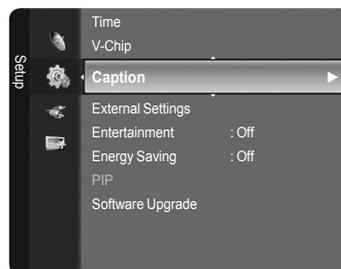
4. Press the **▲** or **▼** button to select "Caption Mode", then press the **ENTER** button. Press the **▲** or **▼** button to select submenu (Default, CC1~CC4 or Text1~Text4) you want, then press the **ENTER** button.
