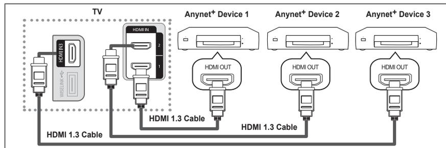
Connect the [HDMI 1], [HDMI 2] or [HDMI 3] jack on the TV and the HDMI OUT jack of the corresponding Anynet+ device using an HDMI cable.
