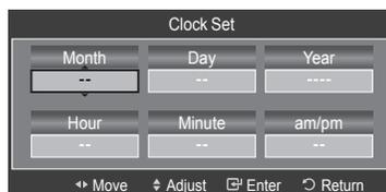
5. Press the **◀** or **▶** button to move to "Month", "Day", "Year", "Hour", "Minute", or "am/pm". Set the date and time you want by pressing the **▲** or **▼** button, then press the **ENTER** button.
