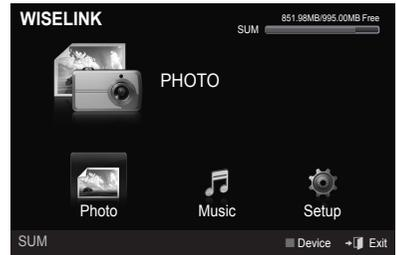
1. Press the **W.LINK** button on the remote control to display the “WISELINK” menu.
