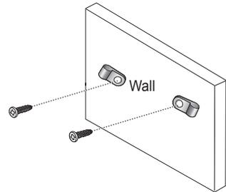
2. Remove the screws from the center back of the TV, put the screws into the clamps, and then fasten the screws onto the TV again.
