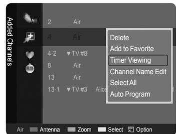
3. Press the **▲** or **▼** button to select "Timer Viewing", then press the **ENTER** button. The Reserve a Program (Timer Viewing) screen appears.
