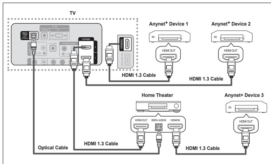
1. Connect the [HDMI 1], [HDMI 2] or [HDMI 3] jack on the TV and the HDMI OUT jack of the corresponding Anynet+ device using an HDMI cable.
