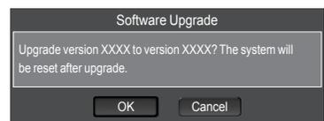
Please be careful to not disconnect the power or remove the USB drive while upgrades are being applied. The TV will turn off and turn on automatically after completing the firmware upgrade. Please check the firmware version after the upgrades are complete. When software is upgraded, video and audio settings you have made will return to their default (factory) settings. We recommend you write down your settings so that you can easily reset them after the upgrade.
