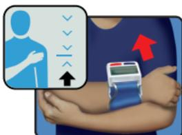
3. Put the arm with the appliance on the other upper arm as shown. Slowly move the hand upward along the upper arm.
