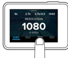
If you select a video resolution (RES) that does not support the frames per second (FPS) setting that is selected, a message appears that instructs you to tap the touch display to automatically move to the FPS setting and select a different value. A similar message appears if you select an FPS that is not supported by the selected resolution.
