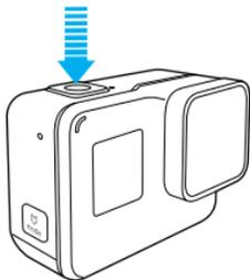
Your camera powers on, beeps several times, and automatically begins capturing video. The camera status lights blink while the camera is recording.
