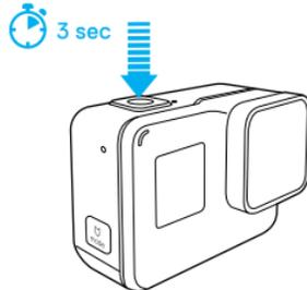
Your camera powers on, beeps several times, and automatically begins capturing time lapse photos. The camera status lights blink once for each photo captured.
