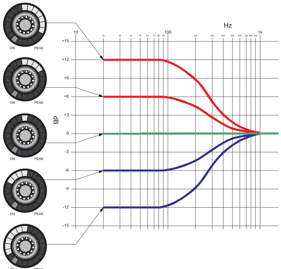
Figure 13: Adjustment range for the BASS function
