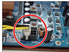
Plugged from a 4-pin ATX12V power.
