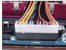
Plugged from a 24-pin ATX12V power.
