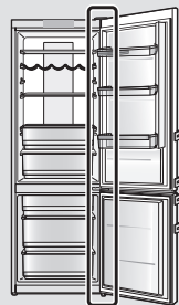
Potential pinch point
