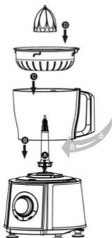
Do not fill the bowl beyond the MAX indication. Built-in safety lock: the citrus press only works when the sieve is assembled properly on the motor unit and the cone is assembled properly in the sieve. All parts have been assembled properly, the cone starts rotating as soon as you turn the switch to the minimum speed setting.
