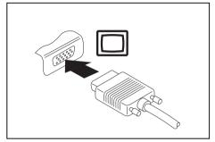
Analogue VGA monitor connection socket
