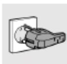
LA PRISE MALE A RELIER AU CABLE D'ALIMENTATION ET LA PRISE MURALE CORRESPONDANTE DOIVENT IMPERATIVEMENT ETRE DE MEME TYPE ET CONFORMES A LA REGLEMENTATION EN VIGUEUR.
