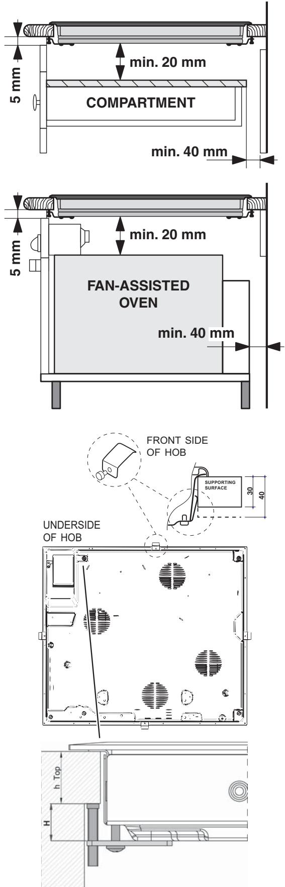
The appliance must be installed on a perfectly level supporting surface.
