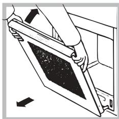
3. Grip the door on the two external sides and close it approximately half way. Pull the door towards you, lifting it out of its slot (*see diagram*). To replace the door, reverse this sequence.
