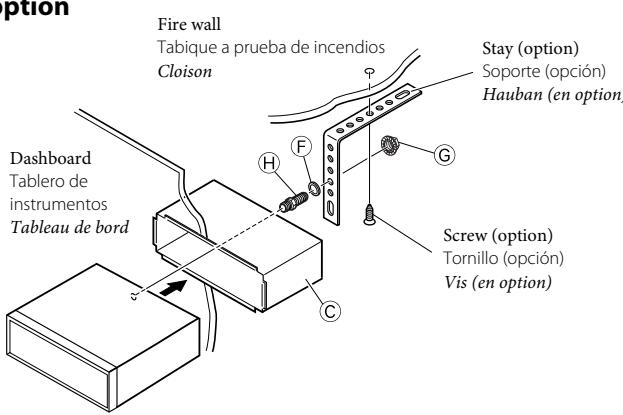
Install the unit at an angle of less than 30°.
