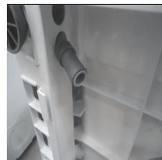
6. Once the machine is in place the feet should be adjusted to ensure that the new hose does not kink when pushing the tumble dryer into position.
