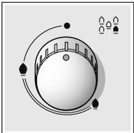
The markings show the position of the corresponding burner and the setting between high and low heat. The flame setting is infinitely variable between high and low.
