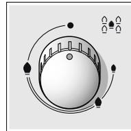
Turning the wok burner control knob beyond the middle flame symbol activates the outer flame ring.
