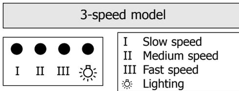
**Note:** If more than one speed button has been depressed, **the hood operates at the fastest.**
