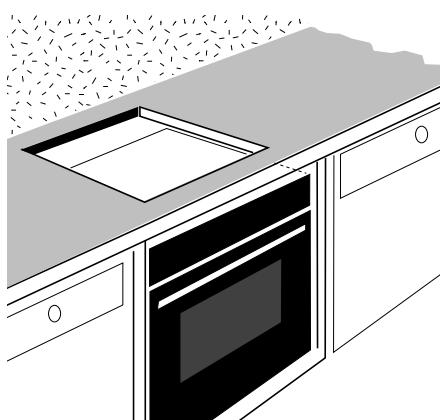
The hob can be fitted directly into the worktop above an oven placed in its upper position (Minimum distance 10 mm).
