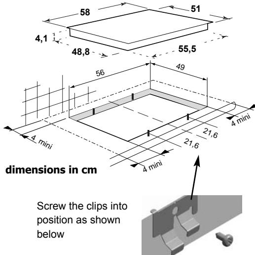
Screw the clips into position as shown below
