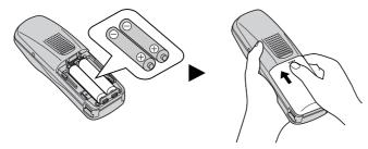
• If the rechargeable batteries are not inserted correctly, the handset will not work.
