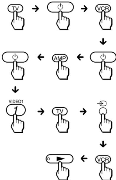
You can programme up to 16 consecutive steps on each of the SYSTEM CONTROL buttons (A – D), including the initial step of pressing switch to a Component Select button.
