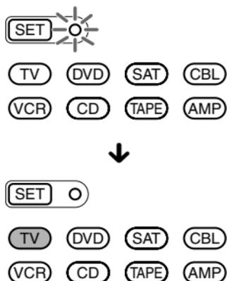
When erasing of a “learned” function is completed, the SET indicator light turns off.
