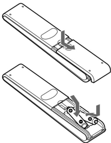
Insert the batteries (negative end first) through the guide clamp within each compartment as shown above.
