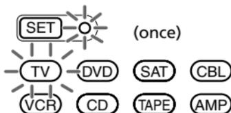
While the Hold function is on, no function can be operated. (The SET indicator and the Component Select button currently selected flash twice.)
