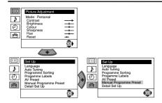
**c)** Normally the automatic fine tuning (AFT) is operating, however you can manually fine tune the TV to obtain a better picture if the picture is distorted.
