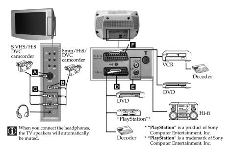
To avoid picture distorsion, do not connect external equipment to connectors A and B at the same time.
