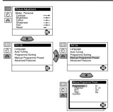
**2** After selecting the **Channel** option, press **\( \rightarrow \)**. Then press  $\bullet$  or  $\bullet$  to select the channel tuning ("C" for terrestrial channels or "S" for cable channels). Next press . After that, press the number buttons to enter directly the channel number of the TV Broadcast or the channel of the VCR signal. If you do not know the channel number, press ◆ or ♠ to search for it. When you tune the desired channel, press **OK** twice to store.
