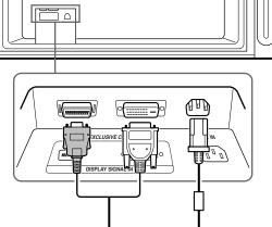
**2** Secure the mains plug to the display's AC IN jack.
