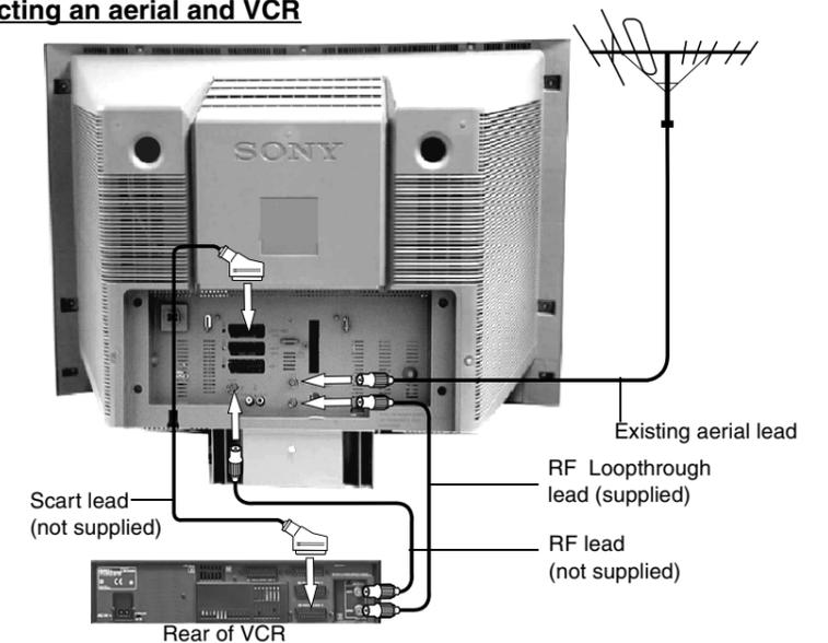
1. Connect your existing aerial lead to the digital socket marked
