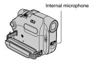
You can record audio by using the internal microphone.
