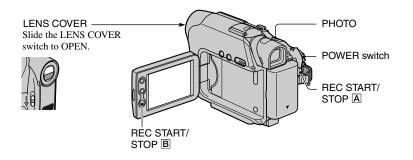
1 Slide the POWER switch in the direction of the arrow to turn on the CAMERA lamp.
