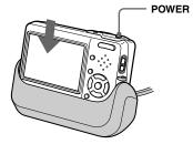
• Make sure the camera is securely connected to the Cyber-shot Station.
