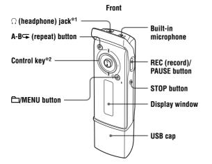
This unit does not have a power on/off switch.
