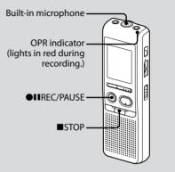
You can record up to 99 messages in each of the four folders (A, B, C, and D). Since a newly recorded message is automatically added behind the last recorded message, you can start recording quickly without searching for the end of the last recording.
