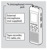
1 Connect a plug-in-power type microphone or other equipment to the \*(microphone) jack.
