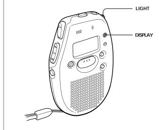
The display changes as follows every time you press DISPLAY. After 10 seconds without pressing any button, the unit returns to clock display.
