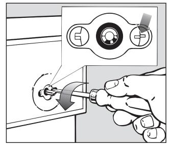
Using a 4-5 mm wide screwdriver turn the adjuster mechanism to the right hand side of the spindle <u>carefully in an anti-clockwise direc-</u> tion until it checks into position.
