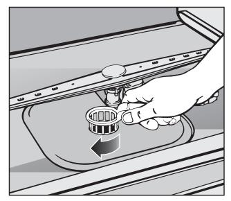
Replace the filter combination so that it lies flat in the base of the wash cabinet. Secure the filter by turning the handle in a clockwise direction.
