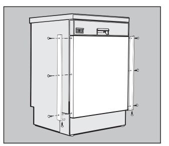
Screw the side decor strips into position.
