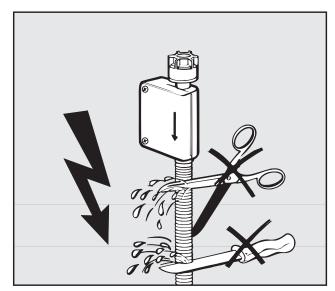
Connect the inlet hose with the "Waterproof-System" preferably vertically (use an angle connector if necessary).
