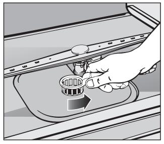
Turn the handle anti-clockwise to release the filters.
