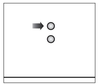
When the salt reservoir is empty the "Salt" indicator light comes on. The reservoir should be refilled with dishwasher salt for reactivation.
