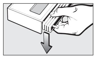
Press out the adapter strips from the fitting slits in the facia panel.
