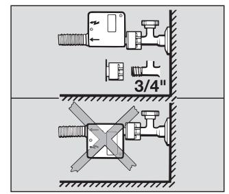
If this is not possible, it can be installed horizontally, but it is essential that the main body of the "Waterproof valve" box is above the hose exit (see illustration). The 'lightning' power symbol should be above the water flow 'arrow'.
