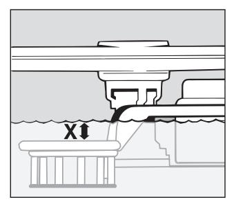
The water level is correct when dimension **"X"** is at least 4 mm.
