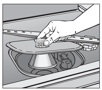
Lift and take the filter combination out of the machine. Remove coarse particles and rinse under running water. Use a nylon brush if necessary.
