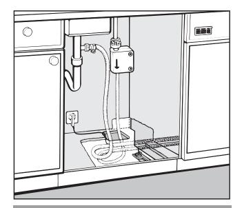
For some installation steps it is necessary to pull the dishwasher slightly out of the recess. Therefore do not make these connections until last. The slides make installation of the dishwasher easier and protect the floor from possible damage when moving the appliance into and out of the recess. They are also used for adjusting the height of the rear screw feet.
