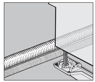
Push the dishwasher right back into the recess. Ensure that drain hose, inlet hose and electric cable are laid to reach the connection point without any kinks.
