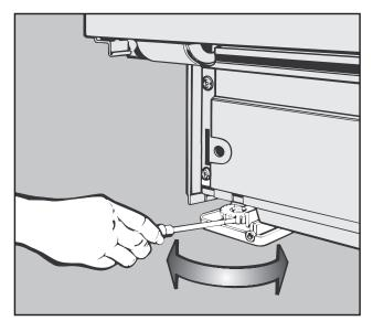
Adjust the <u>front screw feet</u> manually or with a flat blade screwdriver.
