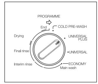
Turn the <u>Programme selector switch</u> (programme sequence indicator) clockwise, until a resistance is felt, to the "start point" of the required programme, e.g. "UNIVERSAL PLUS".
