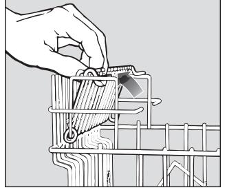
Can either be used for a second row of cups or raised upwards to make room for tall items.
