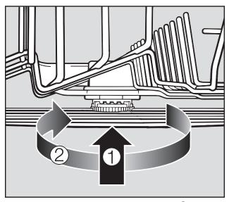
■ Lift up the <u>middle</u> spray arm ① to engage the tooth-wheel mechanism. Then unscrew the spray arm ②.
