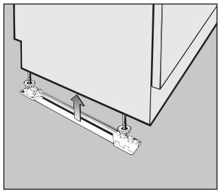
Press the slides - with the ratchet at the rear - under the screw feet.
