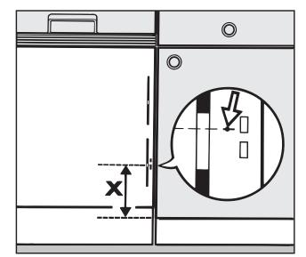
Calculate dimension "X" and make a note of it before attaching the fixing bracket.
