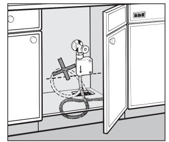
Lay the hose in such a way that it does not rise above the bottom of the "Waterproof" unit casing (see illustration).
