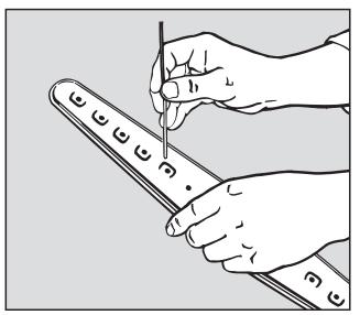
Using a sharp pointed object push the food particles into the spray arm jets and rinse well under running water.
