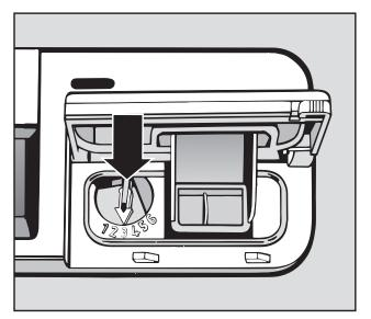
The dosage adjuster (see arrow) in the opening has settings from 1 to 6. It is set to 3 at the factory, as the recommended dose. This setting dispenses approx. 3 ml rinse aid per programme.
