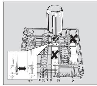
The bottle holder (e.g. for milk or baby bottles) can be used in the bottom basket.
