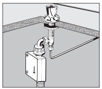
If the stopcock is situated in the worktop, a special angle connector can be ordered from the Miele Spare Parts Dept. (Part No. 2078910).
