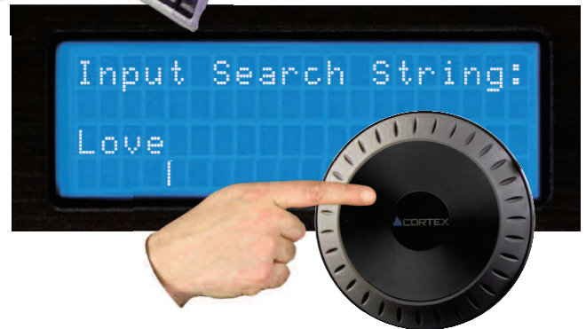
Fig 3.3 - Using Jog Wheel to input a string
