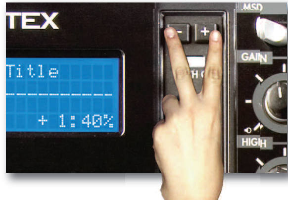
Fig 5.5 - Pitch On/Off by pressing both buttons simultaneously
