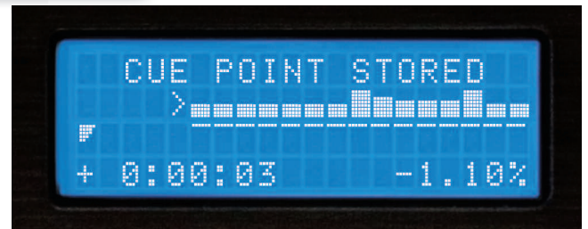
Fig 6.2 - Cue Point Memorization using Shift+Cue
