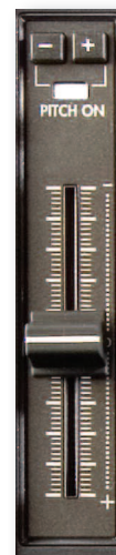
Fig 5.6 - Use either the Pitch control slider the Pitch + & - buttons or the Jog wheel to adjust pitch
