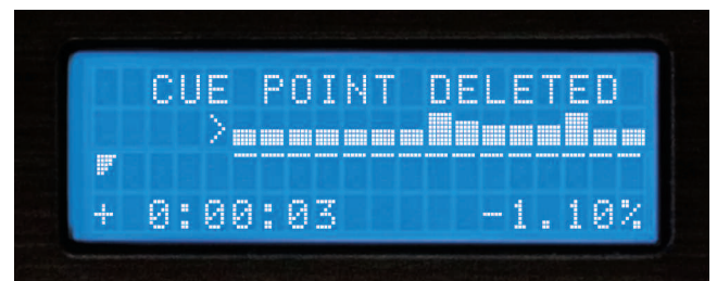
Fig 6.3 - Cue Point Deletion using Shift+Cue
