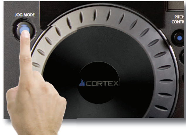
Fig 5.8 - Engaging Jog Mode for FF/REW using the Jog Mode button
