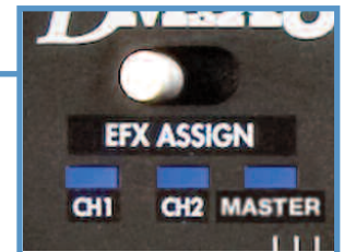
Fig 8.7 Channel assign switch
