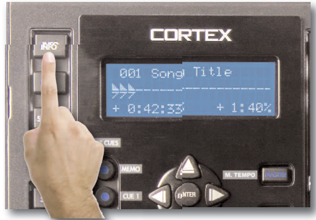
Fig 4.7 - The Info Button is used to display all track attributes
