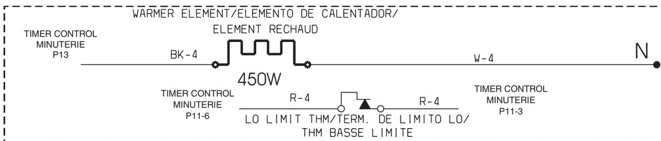
When the Warm and Serve Drawer is first turned on, a "Preheat" circuit is established to provide full power (120 volts). When the temperature at the preheat thermostat reaches 150°F the thermostat opens, and the warmer element starts cycling. If the control is placed on a lower setting, it is possible for the temperature in the drawer to drop enough to allow the preheat thermostat to close again which will allow the element to reenter the "Preheat" mode at full power.
