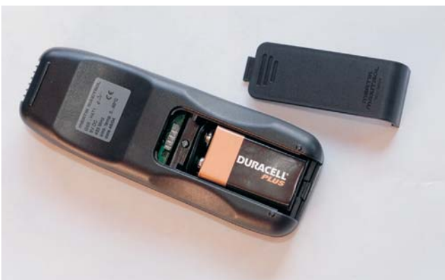
Replacing the batteries in the remote control.
