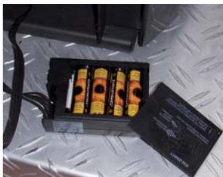
Replacing the batteries of the receiver
