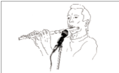
Fig. 5: Microphone placement for the flute.
