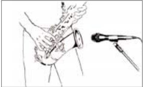
Fig. 6: Microphone placement for the saxophone.
