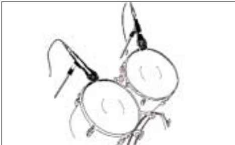
Fig. 10: Microphone placement for tom-toms.
