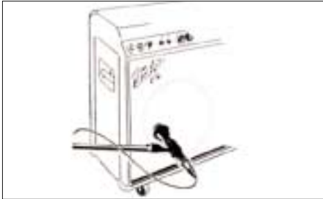
Fig. 9: Microphone placement for a guitar amp.
