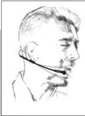
4.2 C 555 L Head-worn Microphone 4.2.1 Positioning the Microphone
