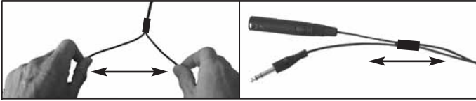
Fig. 2: Separating microphone and headphone cables.
