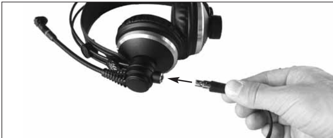
Fig. 1: Plugging the connecting cable into the headset.
